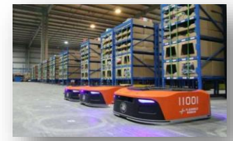
AGVs in smart warehouses Zero packet loss during roaming
